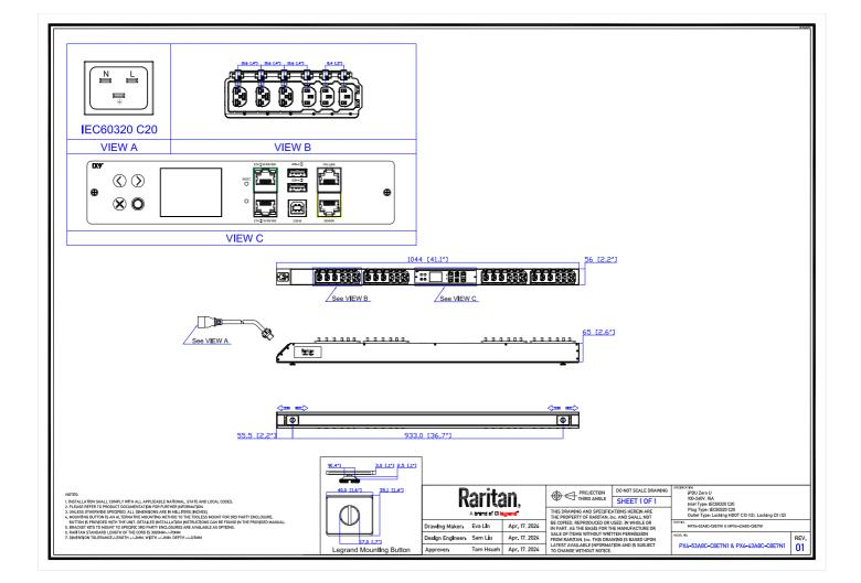
Technical Specifications Model Number: PX4-53A8C-C8E7N1 100-240V, 1Φ, 16/16A, 1.6-3.8kVA
